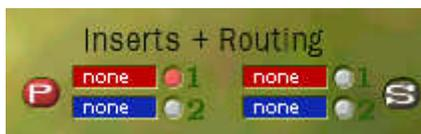
Two effects can be inserted into either the 'Loop' and 'Dry' mixer sections.
